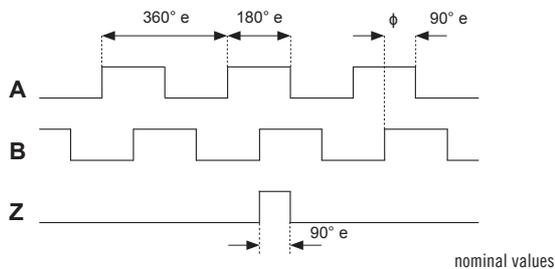
$$\text{Frequency} = \frac{\text{rpm} \times \text{resolution}}{60}$$
