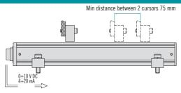
For multi-cursor model, the cursors have to work in the same conditions of distance and temperature. Cursors must be installed on a support made of non-magnetic material (like brass, aluminium or AISI316 stainless steel).
