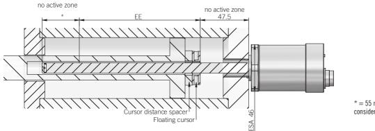
\* = 55 mm up to stroke 1000 mm, from 1250 mm consider 60 mm due to M4 threaded hole
